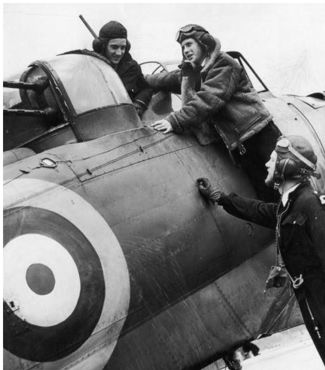
Starboard side of the Roc, notice the cable for the dingy release and one of its "ring-pull" handles, and below it the double cable-run for the anti-spin parachute in the tail.
