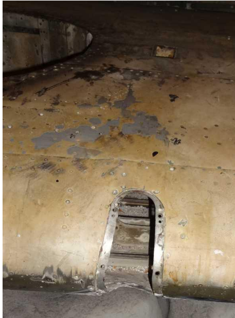
Photo 5: Machine gun opening in wing leading edge, looking from bottom of wing. This area was covered by a plate with only a small hole on the top of the leading edge for the gun to fire through. Presumably this larger opening was required when fitting or removing the gun so it could be angled up through the relatively small access port on top of the wing.
